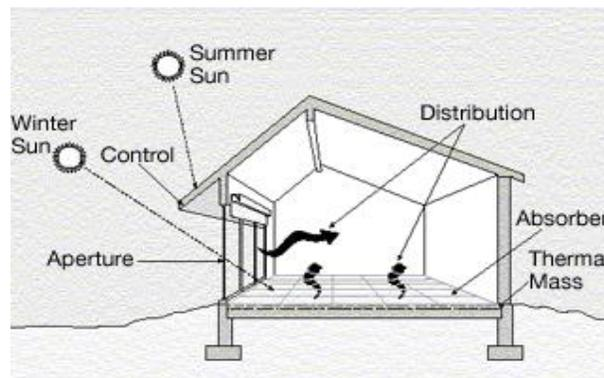
Elements of passive solar design, shown in a direct gain application
