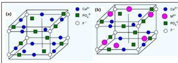
Figure 6. unit cell of apatite mineral (a) before and (b) after interaction with heavy metal ions (M<sup>2+</sup>)
